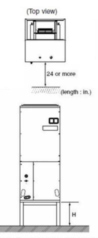
Ensure sufficient space for the bottom of the product (H dimensions) so that a downward slope of 1/100 can be maintained for drain piping, as described for the intake duct installation and in "6. DRAIN PIPING WORK".
