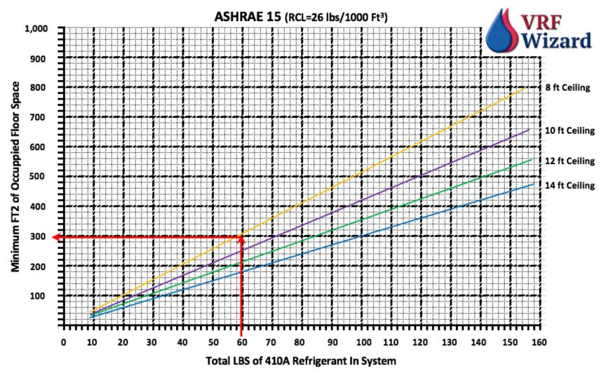
Sample Calculation. Using R401A with a RCL of 26 Lbs./1,000 Ft3 and 60 Lbs. of refrigerant in the system we get the following minimum Ft2 of occupied floor area for an 8 foot ceiling; 288 Ft2
